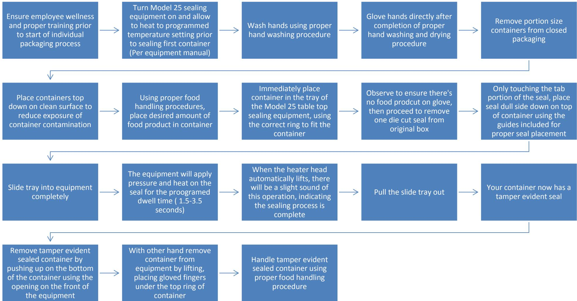
This procedure can be incorporated into any comprehensive HACCP plan. The Wilpack Packaging Tamper Evident Sealing Equipment is a useful tool used to control exposure of contamination or adulteration of food products for human consumption.
