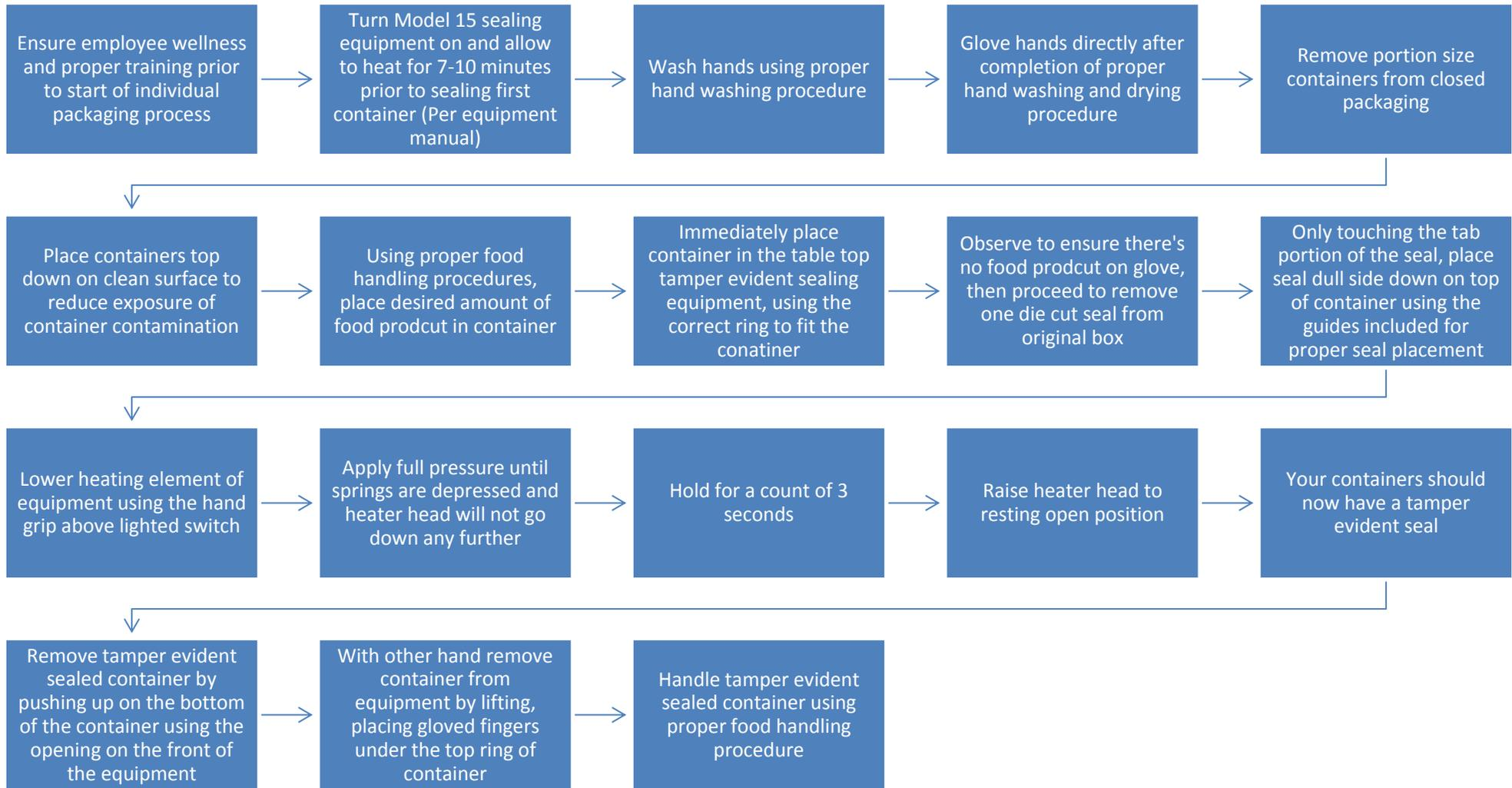
This procedure can be incorporated into any comprehensive HACCP plan. The Wilpack Packaging Tamper Evident Sealing Equipment is a useful tool used to control exposure to contamination or adulteration of food products for human consumption.
